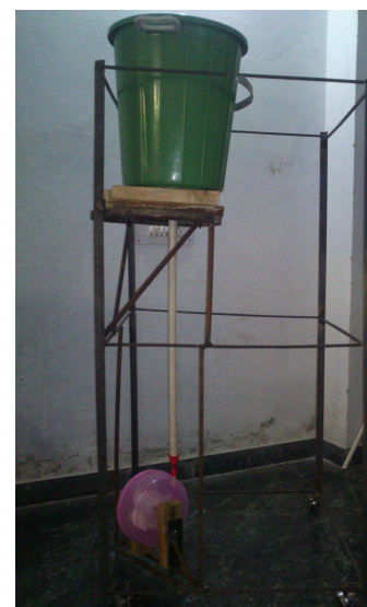
Fig3, Working Model of turbine which producing electricity from wash room waste water.
