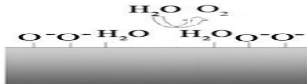
Fig. 3 Schematic Description of the Sensing Mechanism of Water Vapour on the Surface of a Metal Oxide Gas Sensor
