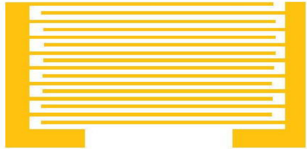
Fig. 7 Microstructure of an Interdigitated Array Electrode
