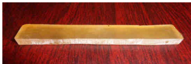
Fig. 2: Bend test specimen for measuring flexural strength
