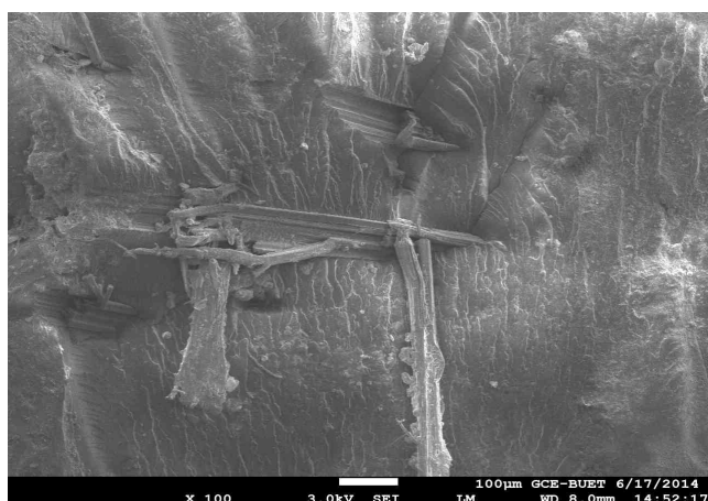
Fig. 5(c): SEM photograph of fracture surface of jute reinforced polyester composite
