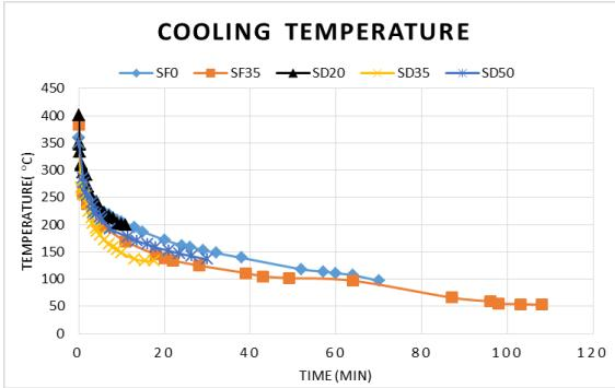
**Fig. 4.Temperature versus time during cooling.**
