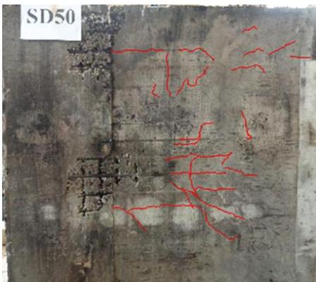
Fig. 8. Cracks pattern for tested slabs.
