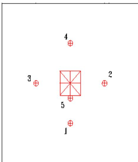
**Fig. 5.**Dial gauges positions.
