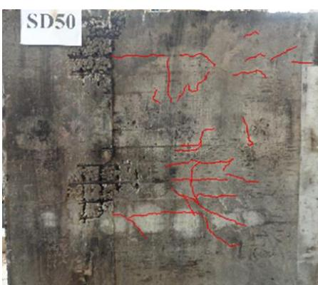
**Fig. 8.**Cracks pattern for tested slabs.
