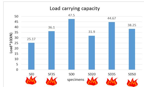
**Fig. 7.**Load carrying capacity for slabs specimens.
