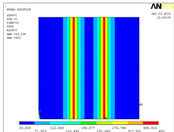
**Fig. 10.** Slab surface temperature after 10 Min.
