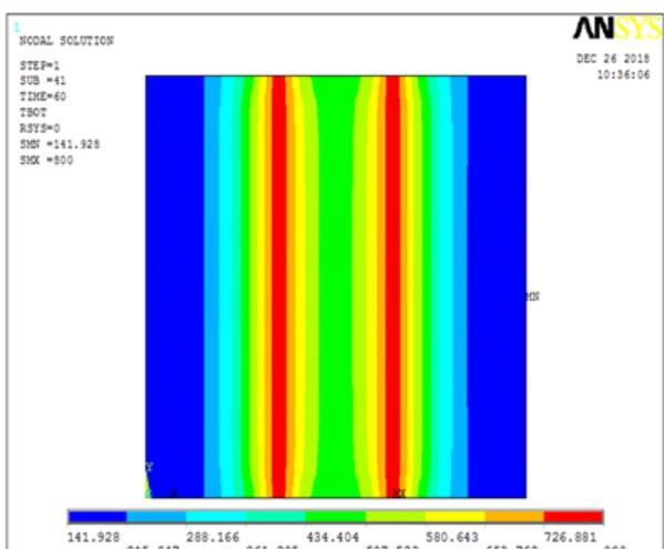
**Fig. 11.** Slab surface temperature after 60 Min.
