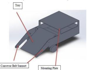
The above figure shows the body of the RC Scrap collection bot. the parts and their function are as follows. Tray: - Used to deliver the Scrap into the Collection Container
