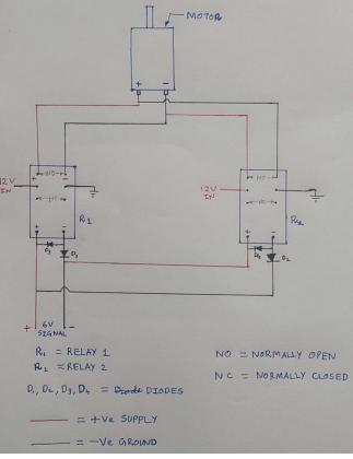
The above circuit is a Motor control Circuit. Here we give a 6 volts DC input signal and depending on the polarity of the signal, the motor at the output changes direction.
