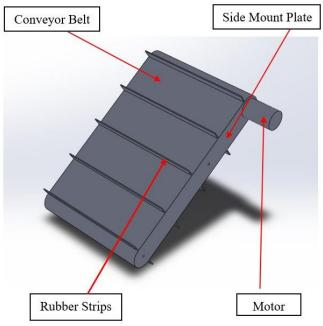
The above figure shows the conveyor belt assembly for collecting the scrap. As the conveyor belt rotates in anti-clock wise direction, the rubber strips fixed to the conveyor belt pulls the scrap onto the tray and into the collection container.
