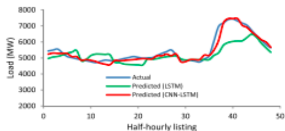
Figure 3. Comparison of Load Forecasting Results of BPS using Different Networks for April 01, 2022
