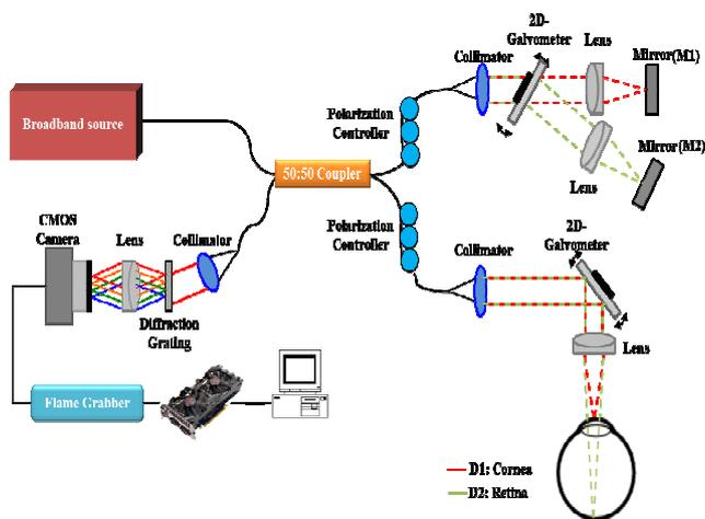
**Figure 1 System Configuration of Optical Switching Mechanism based SD-OCT**
