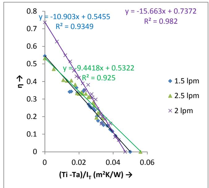
Fig.2. Efficiency curve at three flow rates for Al<sub>2</sub>O<sub>3</sub> - water nanofluid.
