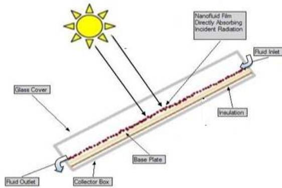
**Fig.1. The schematic of direct absorption solar collector (DASC).**
