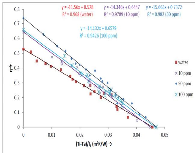
**Fig.3. Efficiency curves for Al<sub>2</sub>O<sub>3</sub>-water nanofluid at different concentrations**
