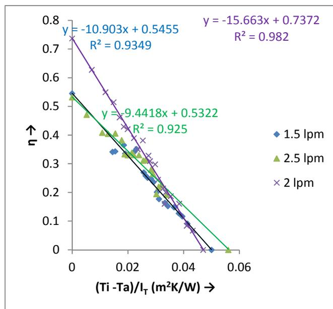
Fig.2. Efficiency curve at three flow rates for Al<sub>2</sub>O<sub>3</sub> - water nanofluid.
