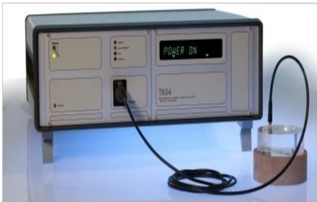
Fig 1. shown above is equipment for measuring thermal conductivity
