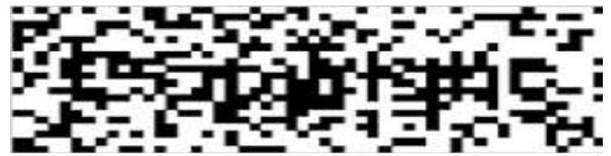
Figure 3 (A) - 5% Gaussian Noise (k = 5)
