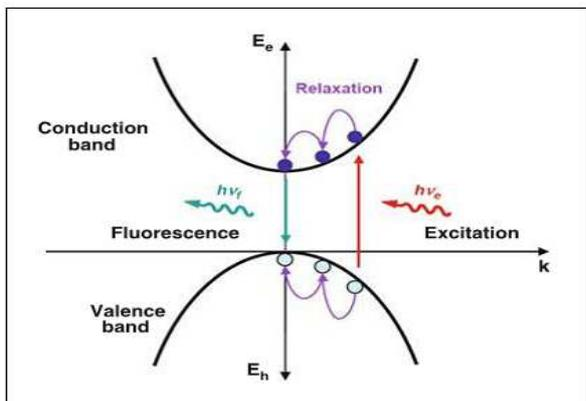
Figure I.5 Fluorescence in bulk semiconductor
