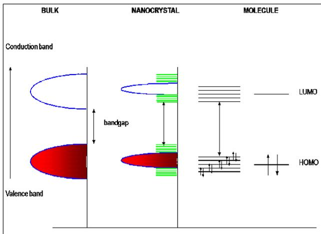
**Figure I.3 Band structure of nanocrystal compared with that of bulk semiconductor**
