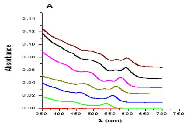
**Figure I.4 Absorption spectra of CdSe semiconductor nanocrystals showing size tunability**
