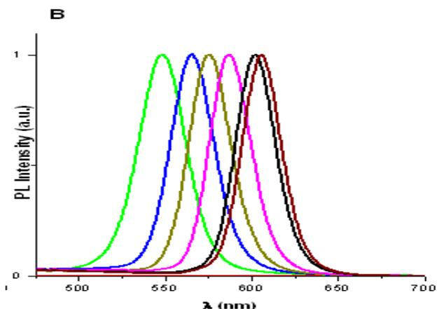
Figure I.6 Fluorescence spectra of CdSe semiconductor nanocrystals showing quantum confinement and size tunability. [1]
