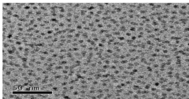
**Figure I.2** Spherical semiconductor nanocrystals. (TEM micrograph of CdSe quantum dots)
