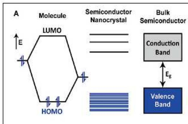
**Figure I.1** Electronic energy states of a semiconductor in the transition from discrete molecules to the nanosized crystal and bulk crystals. Blue shading denotes ground state electron occupation
