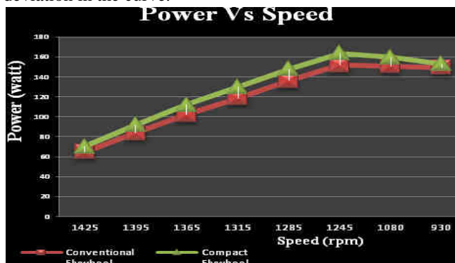
Fig. 7 Graph of Power Vs Speed of Conventional Flywheel and Compact Flywheel
