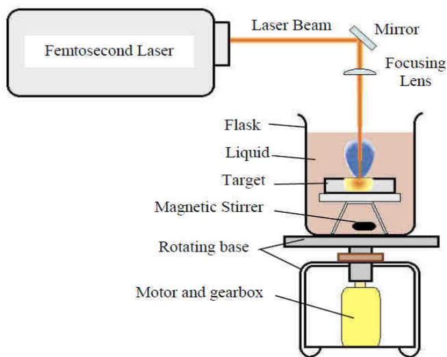
Fig. 1 The set up experiment of femtosecond laser ablation
