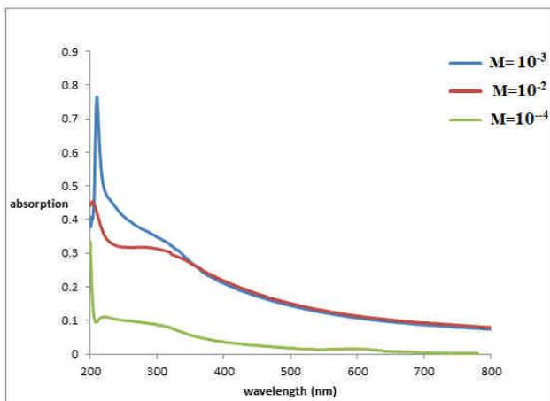
**Fig. 2 UV–visible absorption spectra of ZnO nanoparticles prepared in different values of CTAB molarity ( $\lambda$  800 nm, E = 0.5 mJ/pulse,)**
