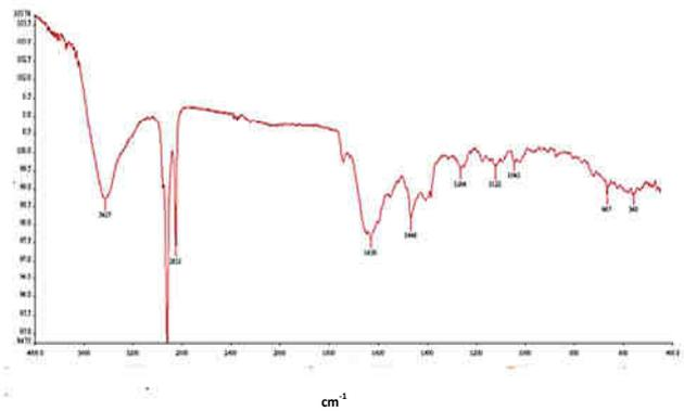
**Fig. 3 FTIR spectra of ZnO nanoparticles prepared in CTAB Media ( $\lambda$  = 800 nm, E = 0,5 mJ/pulse)**
