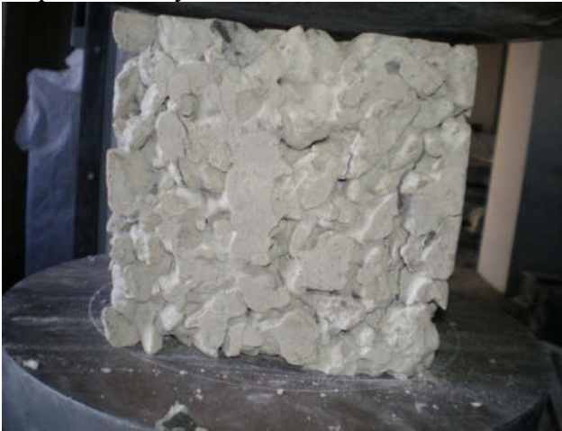
Figure 5: Test specimen for compressive Strength test
