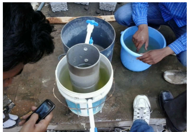
Figure 4: Constant head water permeability test
