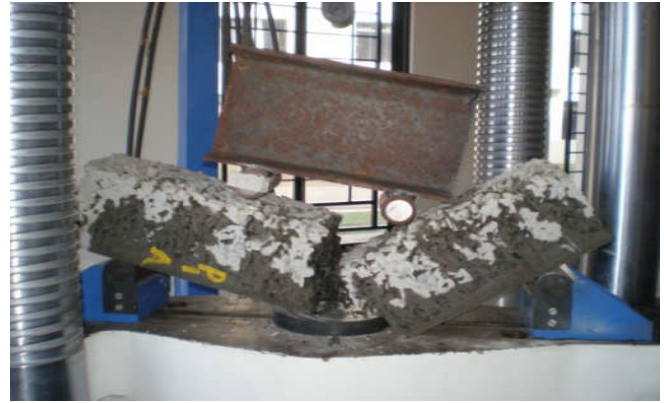
Figure 9: Flexural failure of beam section
