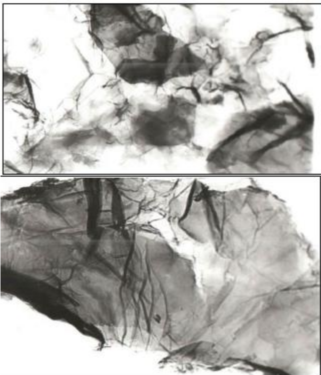
Figure 5. TEM images of graphene oxide (GO) sheets obtained by a modified Hummer's method.
