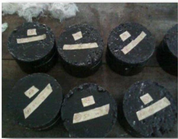
Fig.3.1 Sample for Marshal Stability Test
