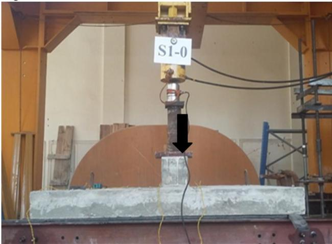
Fig. 2. Test Set-up for loading slabs.
