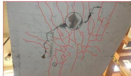
**Fig. 11. Crack pattern and mode of failure S6-50.**
