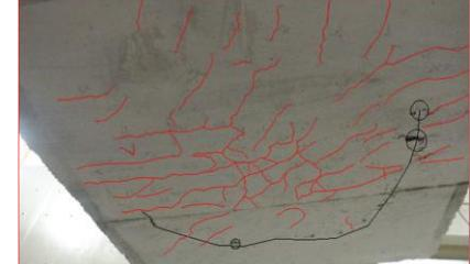
**Fig. 13. Crack pattern and mode of failure S7-70.**
