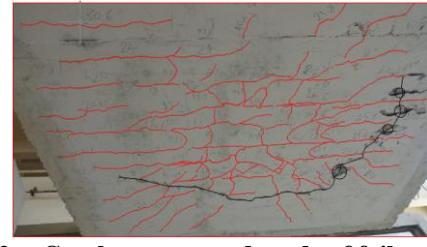
**Fig. 12. Crack pattern and mode of failure S5-60.**
