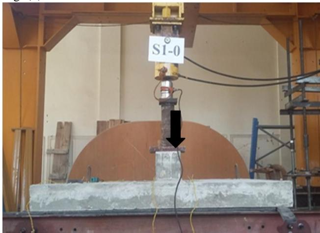
**Fig. 2.Test Set-up for loading slabs.**
