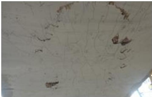
**Fig. 7. Crack pattern and mode of failure S1-0.**
