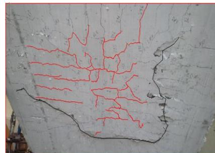
**Fig. 10. Crack pattern and mode of failure S3-35.**
