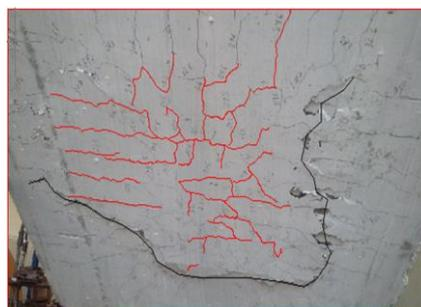
Fig. 10. Crack pattern and mode of failure S3-35.
