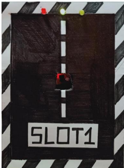
Fig. 12. Green LED glows when slot is empty
