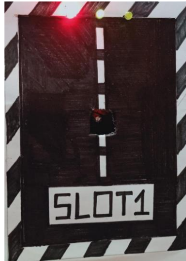
Fig. 14. Red LED glows when slot is booked by user through app
