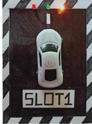
Fig. 13. Yellow LED glows when slot is occupied
